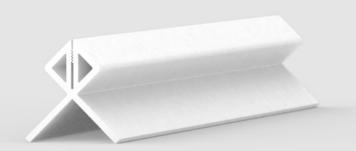
The Modular Corner Load joins the fabric at outside corners. The fabric sits tightly in between the teeth of the track. The teeth are serrated downwards to keep the fabric from slipping out. The track features an anti-warp feature to prevent an imprint on the fabric, and also an anti-slip feature to adhere better to surfaces. Taller tracks have additional support structures added to reinforce stability.
